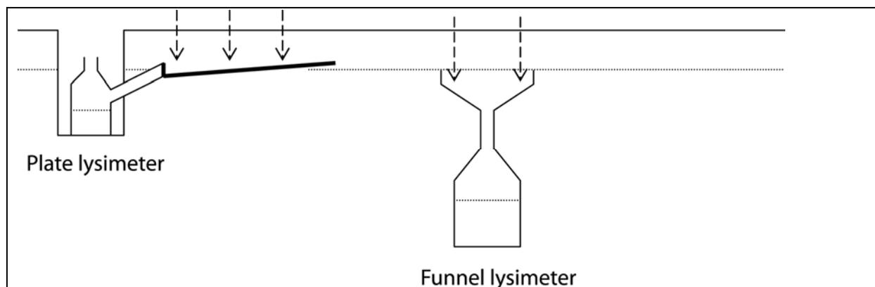
**Figure 2: Examples of different types of zero-tension lysimeters**
