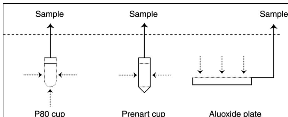
**Figure 1: Examples of different types of tension lysimeters**
