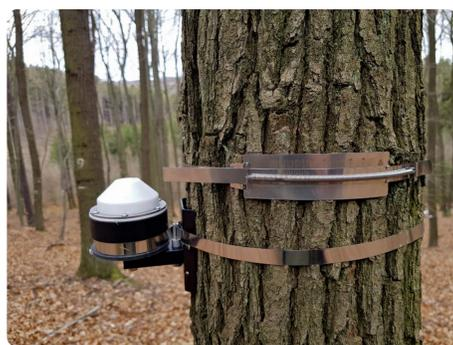
Fig 1 Girth band DB20 (above) and electronic band dendrometer DRL26 (below)
