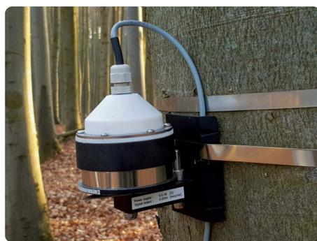
Fig 2 Electronic band dendrometer DR26
