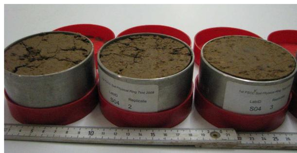
**Photo 4: Three sampling rings of lab S04 showing cracks by disturbance**
