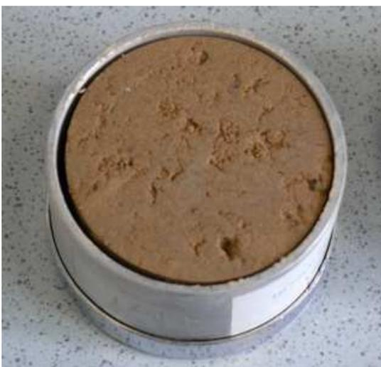
**Photo 3: One sampling ring of lab P11 where the soil shrunk during transport**
