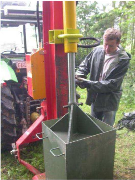
**Photo 1: Hydraulic compression system driven by the PTO of a tractor**
