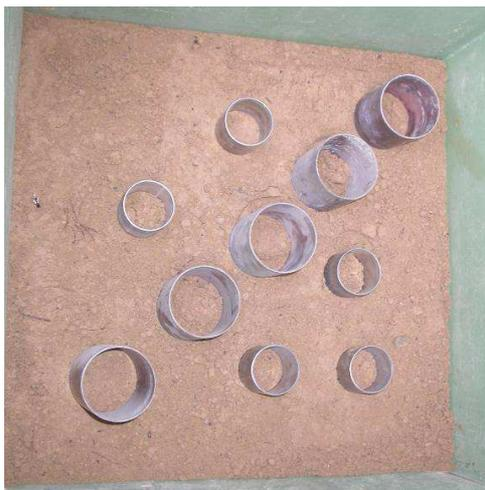
Photo 5: Homogeneity tests in the containers
