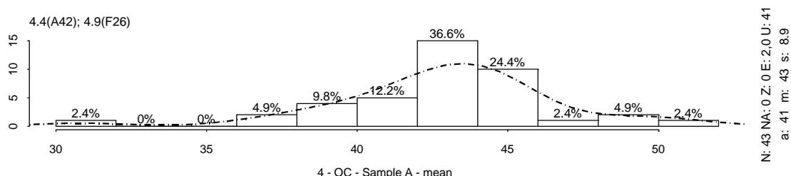
**Figure 1: Histogram showing relative percentages and a rescaled density curve of the mean of three replicates of the measured parameter 'total organic carbon' in Sample A. The units of the X-axis are in g/kg.**
