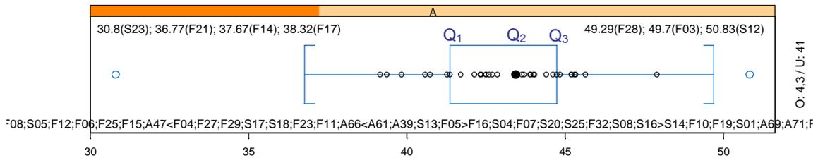
**Figure 2: Box plot of the mean values reported for sample A for 'total organic carbon'. The units of the X-axis are in g/kg.**
